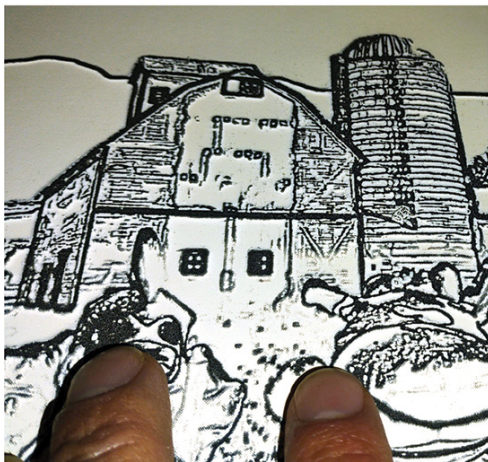
Figure 3: High tech approaches to making tactile graphics include microcapsule or “swell” paper. Swell paper is coated with particles that expand when heated. It can be printed or drawn on in grayscale, then swollen using a heat lamp that will heat the darker regions faster than the light. This graphic was made by P7, who designed the graphic and solicited help from the library which had a swell machine to reproduce it tactilely. The graphic includes a photo of a farm and ranch scene with raised print and braille.
